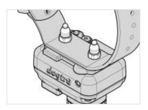
The collar should be fitted so that the Surgical Stainless Steel contact points press firmly against the dog's skin.
