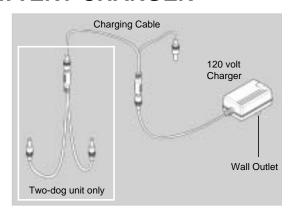
The battery charger and charging cables allow you to charge both the transmitter and receiver at the same time. The battery charger is designed for a 120-volt wall outlet. (European 230-volt AC chargers and 12-volt field charger for Lithium-Polymer batteries for your automobile are also available.)
